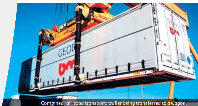
Combined rail-road transport: trailer being transferred to a wagon.
